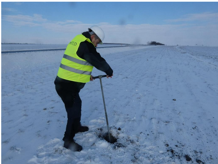
Photo 2.31. Soil sampling at a depth of 30 cm - monitoring point P9
