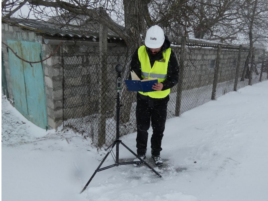
Photo 2.19. Noise level measurement at a sensitive receptor - monitoring point P6
