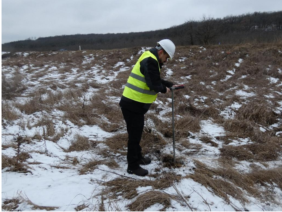
Photo 2.46. Soil sampling at a depth of 30 cm - monitoring point P14
