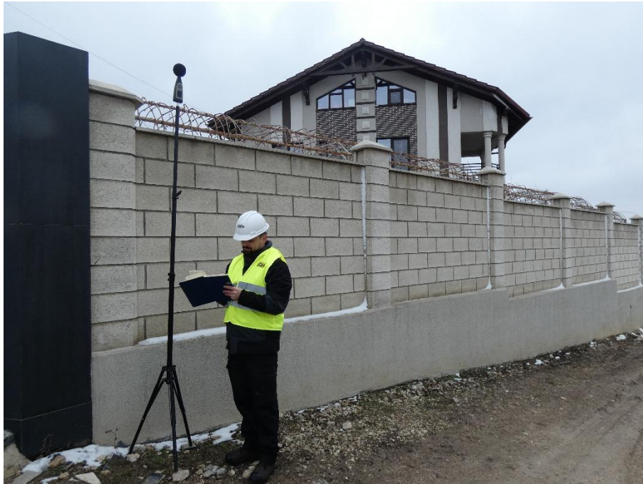
Photo 2.52. Noise level measurement at a sensitive receptor - monitoring point P16
