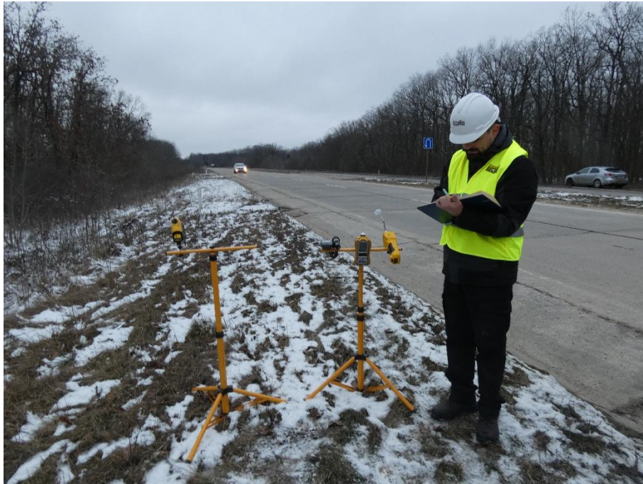
Photo 2.42. Air sampling and measurement - imissions: NO 2 and SO 2 , particulate matter PM 10 , volatile organic compounds (VOCs), and meteorological conditions - P13 monitoring point
