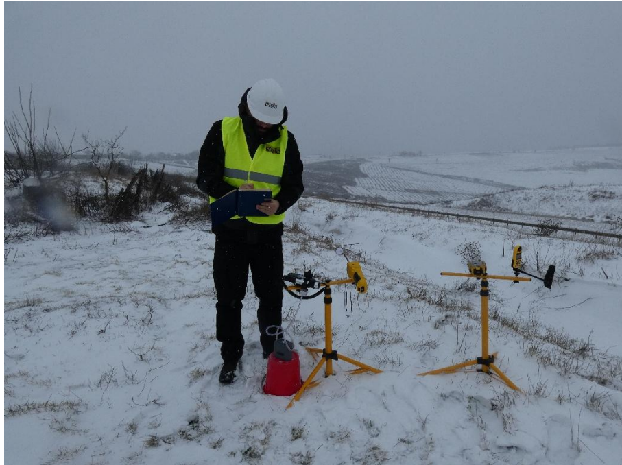
Photo 2.33. Air sampling and measurement - imissions: pollutants - NO, NO 2 , SO 2 , CO and CH 4 , particulate matter PM 2.5 , PM 10 and PM total , volatile organic compounds (VOCs) and measurement of meteorological conditions - monitoring point P10
