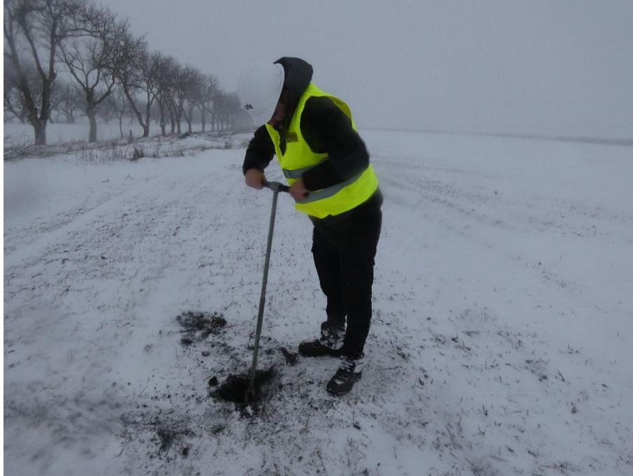
Photo 2.22. Soil sampling at a depth of 30 cm - monitoring point P6
