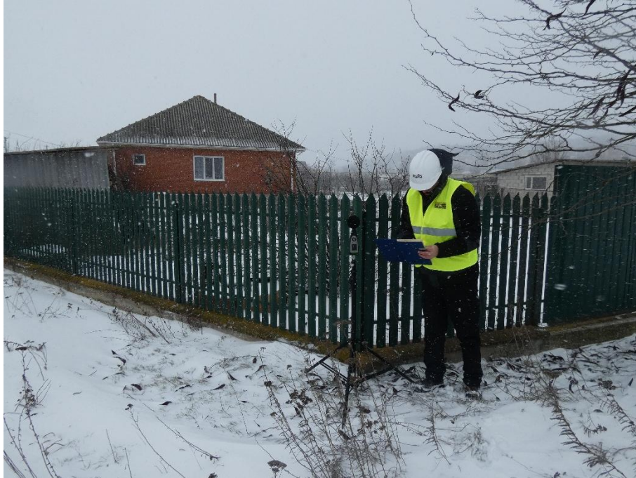
Photo 2.25. Noise level measurement at a sensitive receiver - monitoring point P7
