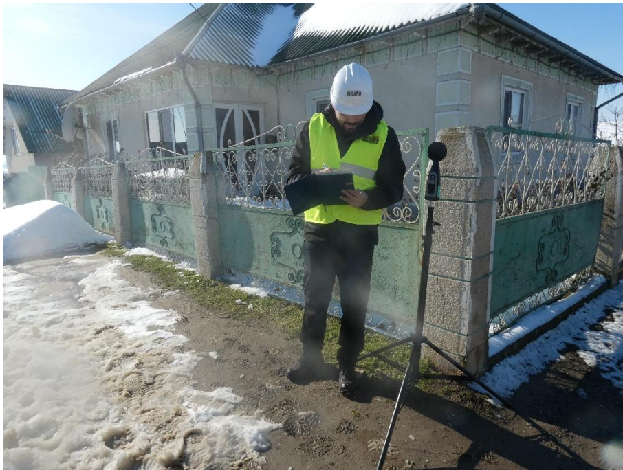
Photo 2.13. Noise level measurement at a sensitive receptor - monitoring point P3
