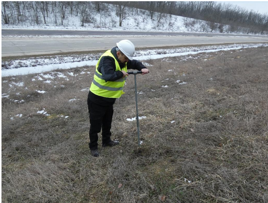
Photo 2.39. Soil sampling at a depth of 5 cm - monitoring point P12
