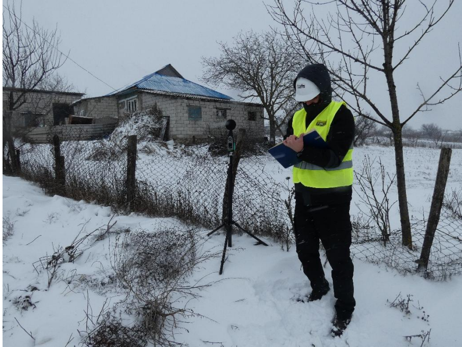
Photo 2.34 . Noise level measurement at a sensitive receptor - monitoring point P10
