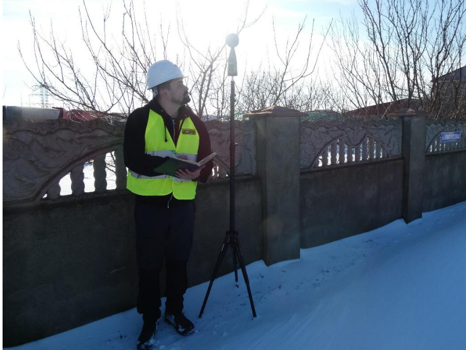
Photo 2.9. Noise level measurement at a sensitive receiver - P2 monitoring point
