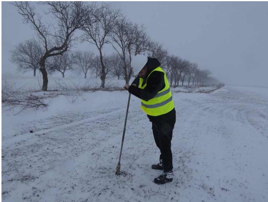
Photo 2.21. Soil sampling at a depth of 5 cm - monitoring point P6
