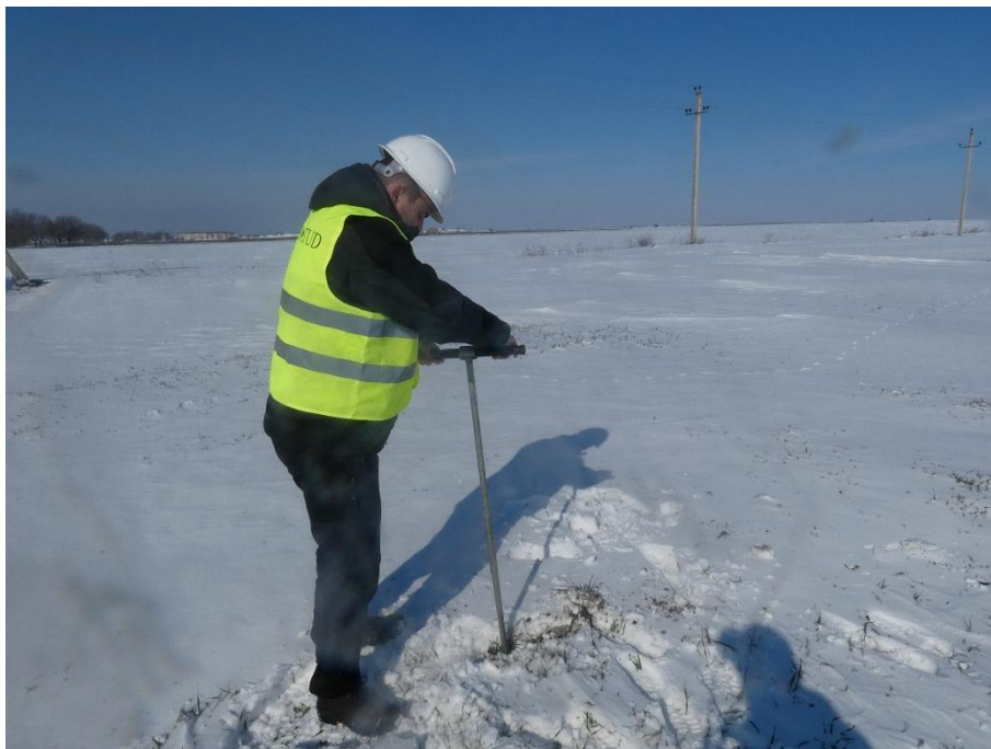
Photo 2 .15 . Soil sampling at a depth of 5 cm - monitoring point P4
