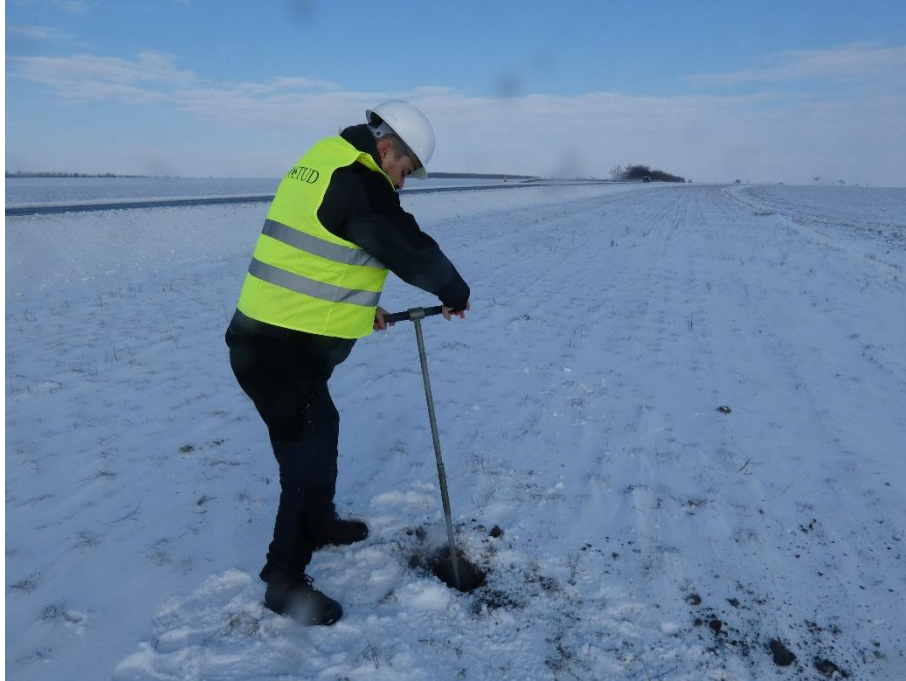
Photo 2.28. Soil sampling at a depth of 30 cm - monitoring point P8
