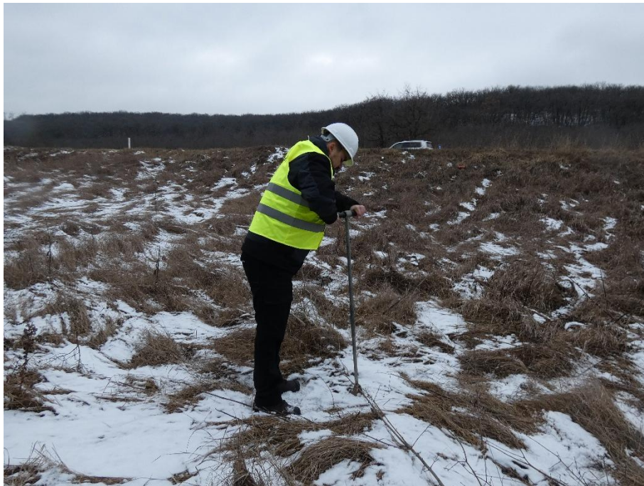
Photo 2.45. Soil sampling at a depth of 5 cm - monitoring point P14
