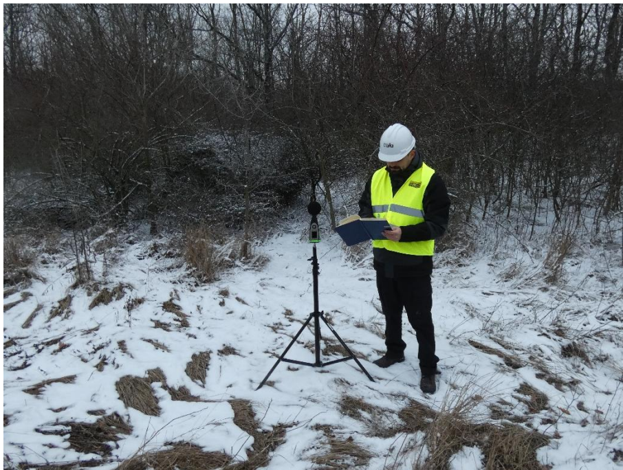
Photo 2.43. Noise level measurement - monitoring point P13
