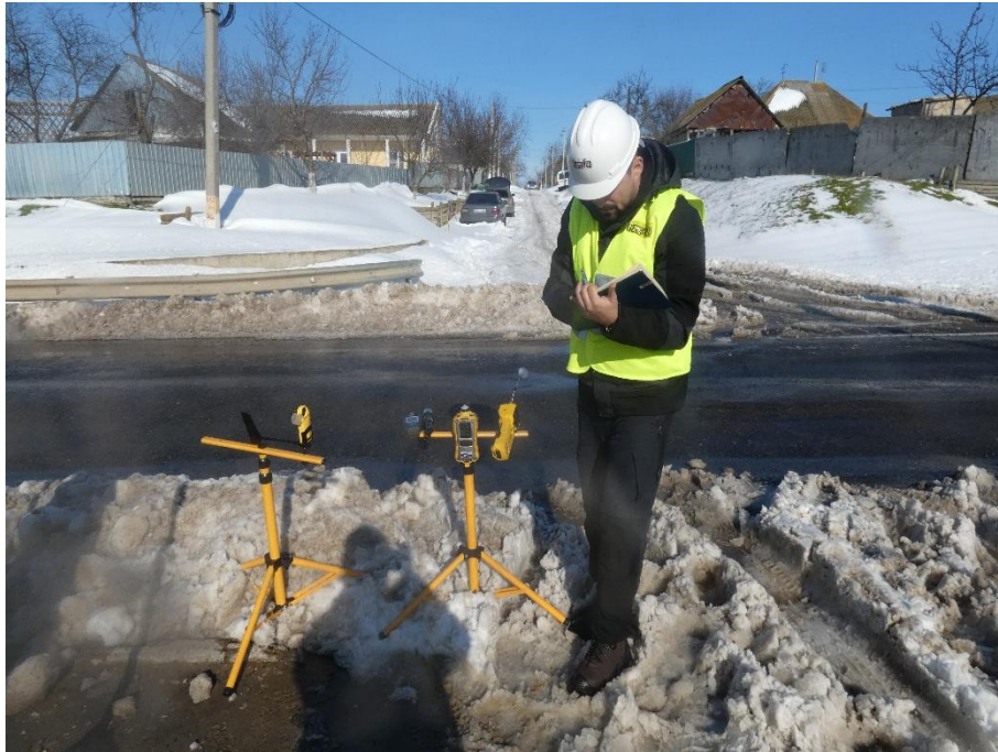
Photo 2.12. Air sampling and measurement - imissions: pollutants - NO, NO 2 , SO 2 , CO, and CH 4 , particulate matter PM 2.5 , PM 10 and PM total , volatile organic compounds (VOCs), and measurement of meteorological conditions - monitoring point P3
