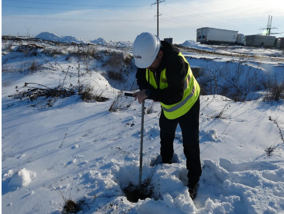
Photo 2.6 . Soil sampling at a depth of 30 cm - monitoring point P1
