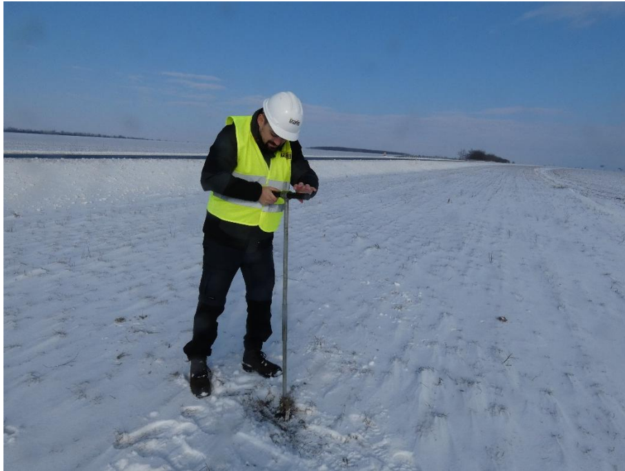
Photo 2.30. Soil sampling at a depth of 5 cm - monitoring point P9
