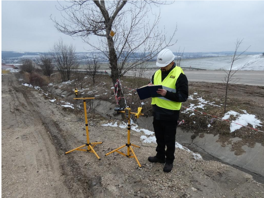
Photo 2.51. Air sampling and measurement – imissions: pollutants – NO, NO 2 , SO 2 , CO, and CH 4 ; particulate matter PM 2.5 , PM 10 , and PM total; volatile organic compounds (VOCs) and measurement of meteorological conditions - monitoring point P16
