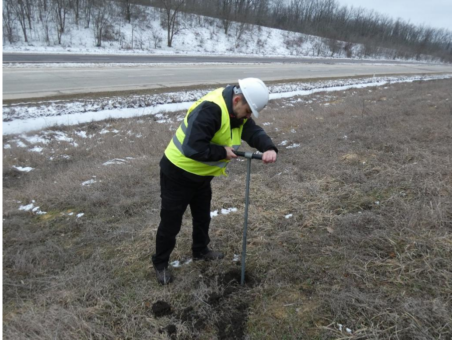
Photo 2.40. Soil sampling at a depth of 30 cm - monitoring point P12
