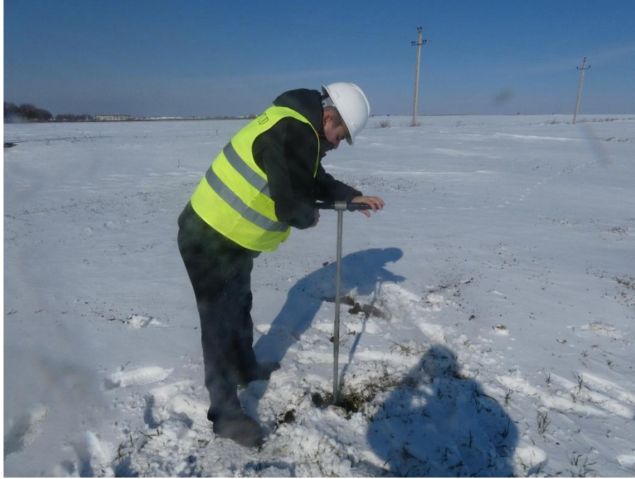
Photo 2 .16 . Soil sampling at a depth of 30 cm - monitoring point P4
