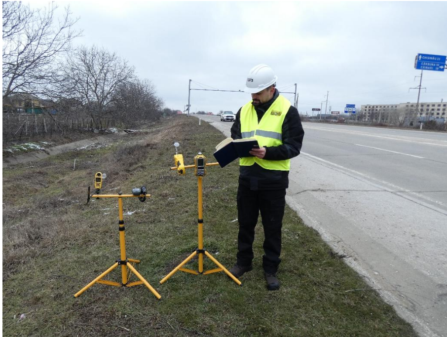
Photo 2 .48 . Air sampling and measurement - imissions: pollutants - NO, NO 2 , SO 2 , CO, and CH 4 , particulate matter PM 2.5 , PM 10 and PM total , volatile organic compounds (VOCs) and measurement of meteorological conditions - monitoring point P15
