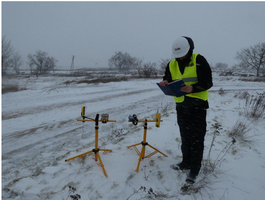
Photo 2.24. Air sampling and measurement - imissions: pollutants - NO, NO 2 , SO 2 , CO, and CH 4 , particulate matter PM 2.5 , PM 10 and PM total , volatile organic compounds (VOCs) and measurement of meteorological conditions - monitoring point P7
