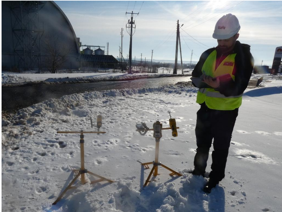
Photo 2.2. Air sampling and measurement – imissions: pollutants—NO, NO 2 , SO 2 , CO, and CH 4 , particulate matter PM 2.5 , PM 10 and PM total , volatile organic compounds (VOCs) and measurement of meteorological conditions - monitoring point P 0
