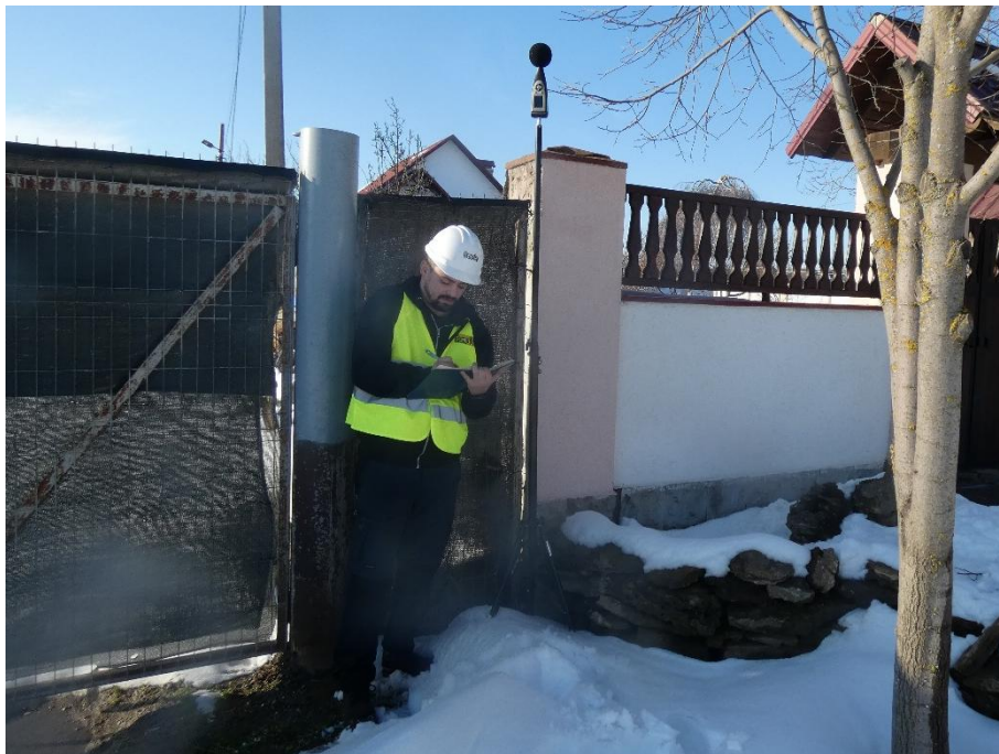
Photo 2.3. Noise level measurement at a sensitive receptor - monitoring point P 0
