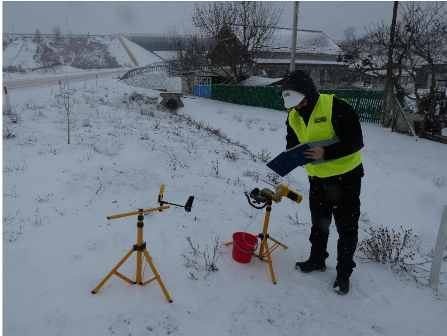
Photo 2.36. Air sampling and measurement – imissions: pollutants – NO, NO 2 , SO 2 , CO, and CH 4 ; particulate matter PM 2.5 , PM 10 and PM total; volatile organic compounds (VOCs) and measurement of meteorological conditions - monitoring point P11
