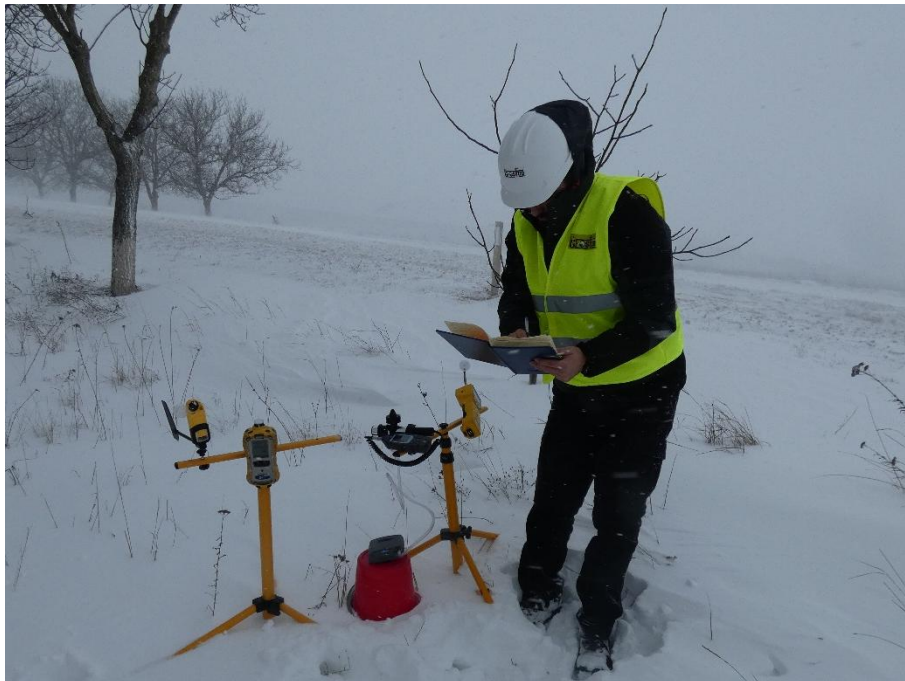
Photo 2.18. Air sampling and measurement – imissions: pollutants – NO, NO 2 , SO 2 , CO, and CH 4 ; particulate matter PM 2.5 , PM 10 , nd PM total; volatile organic compounds (VOCs) and measurement of meteorological conditions - monitoring point P5
