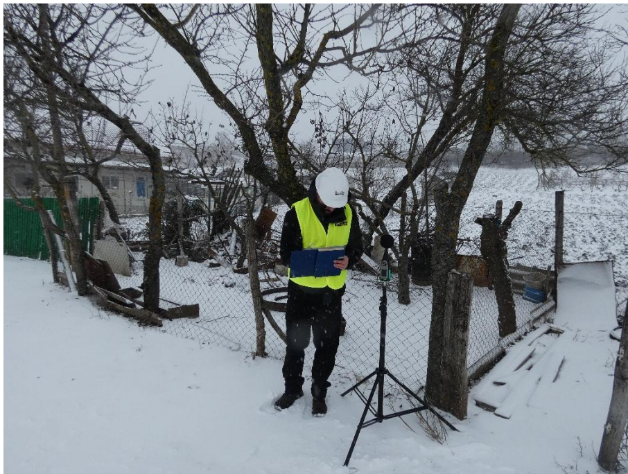
Photo 2.37. Noise level measurement at a sensitive receptor - monitoring point P11
