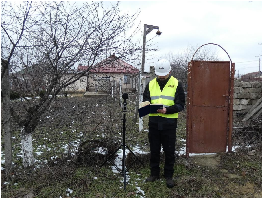
Photo 2.49. Noise level measurement at a sensitive receptor - monitoring point P15
