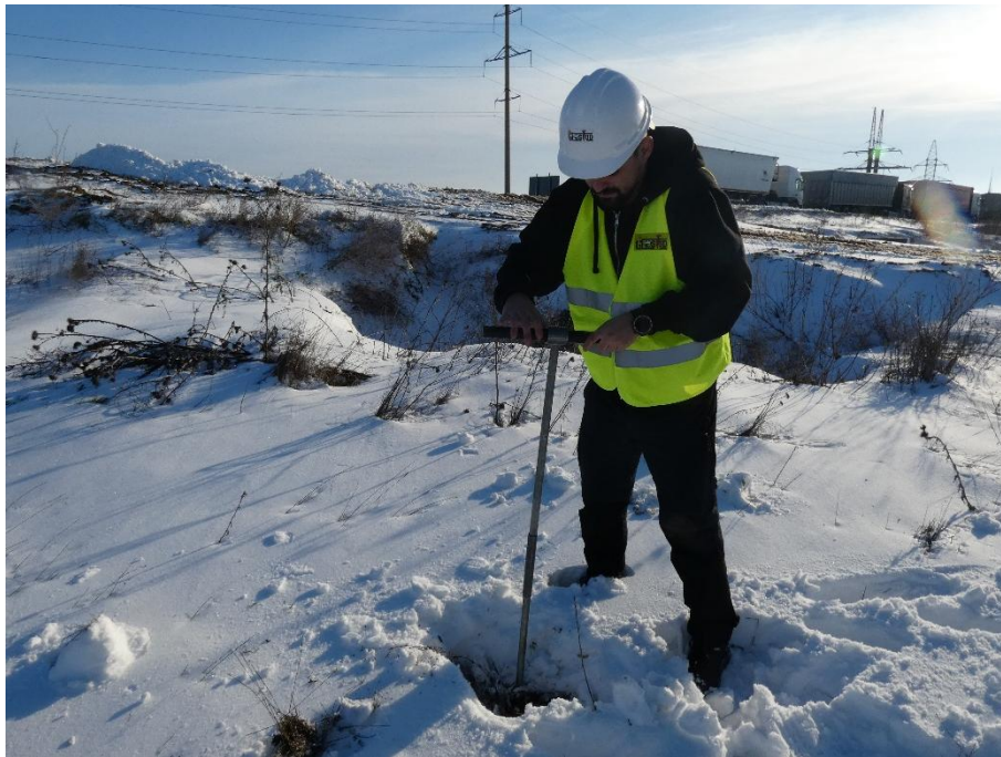
Photo 2.5. Soil sampling at a depth of 5 cm - monitoring point P1
