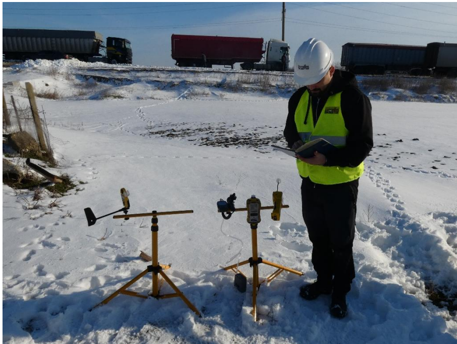
Photo 2.8. Air sampling and measurement - imissions: pollutants - NO, NO 2 , SO 2 , CO, and CH 4 , particulate matter PM 2.5 , PM (10) and PM total , volatile organic compounds (VOCs) and measurement of meteorological conditions - monitoring point P2
